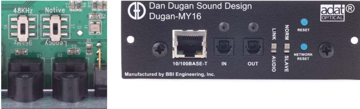
**Figure 2-1** Circuit board and rear panel switches
