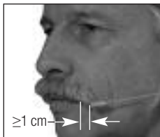
Fig. 9: Microphone capsule position for optimum audio.
