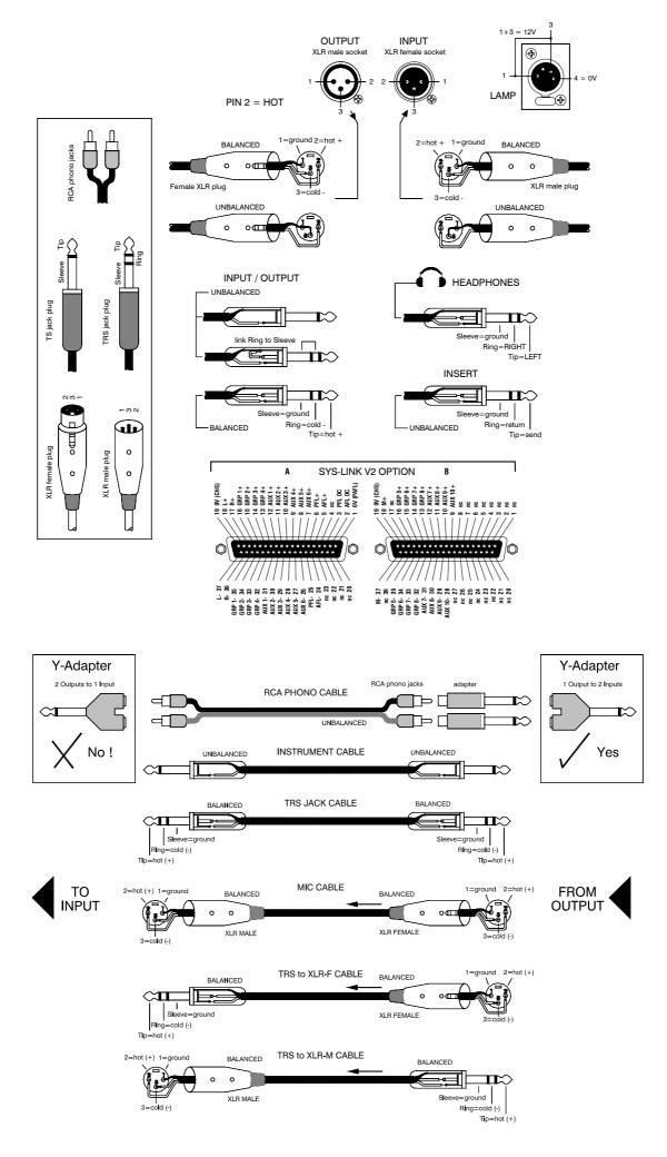
The GL2800 uses professional grade 3 pin XLR and 1/4" TRS (3 pole) jack sockets. To ensure best performance, we recommend that you use high quality audio cables and connectors, and take time to check for reliable and accurate cable assembly. It is well known that most audio system problems are due to faulty or sub standard interconnecting leads. The following plugs may be used to connect audio to the console:
