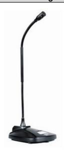
**Set up and position the microphones** - It is best to use the same type of microphone and position them so that the speaking participants are not too close or too far from each mic. To avoid false triggering and phasing set the distance from each voice to mic to be closer than the distance between the mics. The distances from each mic to voice should be similar for consistent operation.
