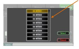
**Multitrack Record** – You can record to a USB storage device plugged into Qu-Drive:
