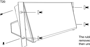
Secure Qu-SB into the rack using the 2x M6x16 screws (AB10301) and washers (AB0345).
