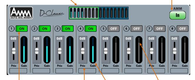
**ON/OFF** – Touch to turn on the channels you want to be affected by the AMM. The AMM sets the channel fader to '0', takes over gain control and lights the gain meter.
