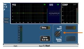
**Insert** switches an internal FX in or out if one has been patched into the mix. The button is disabled when the insert is not patched. The FX is inserted at the start of the processing before the EQ.
