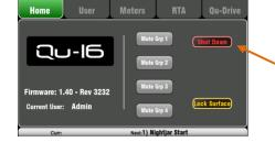
**Switching the mixer off** – First select the **Home** screen. Touch **Shut Down** to safely complete processes such as parameter storing and USB data transfer or recording. Once complete, press the ON/OFF switch to turn the mixer off.
