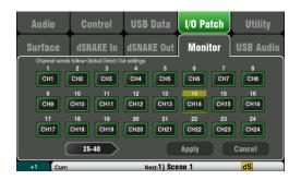
This screen presents the patching of the dSNAKE remote monitor audio outputs. This allows the Qu mixer to work with the Allen & Heath **ME Personal Monitor** mixing system.
