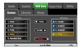
Individual Scenes can be transferred between Qu mixers via a USB device (key or drive) plugged into the Qu-Drive port. This provides a quick way to transfer settings without overwriting the current scenes and preferences.
