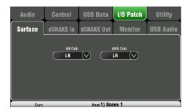
Use this screen to patch signals to the rear panel Alt Out and AES outputs. Touch a box to open up the list of available options. Changes are applied instantly. You can also touch outside the list to exit.
