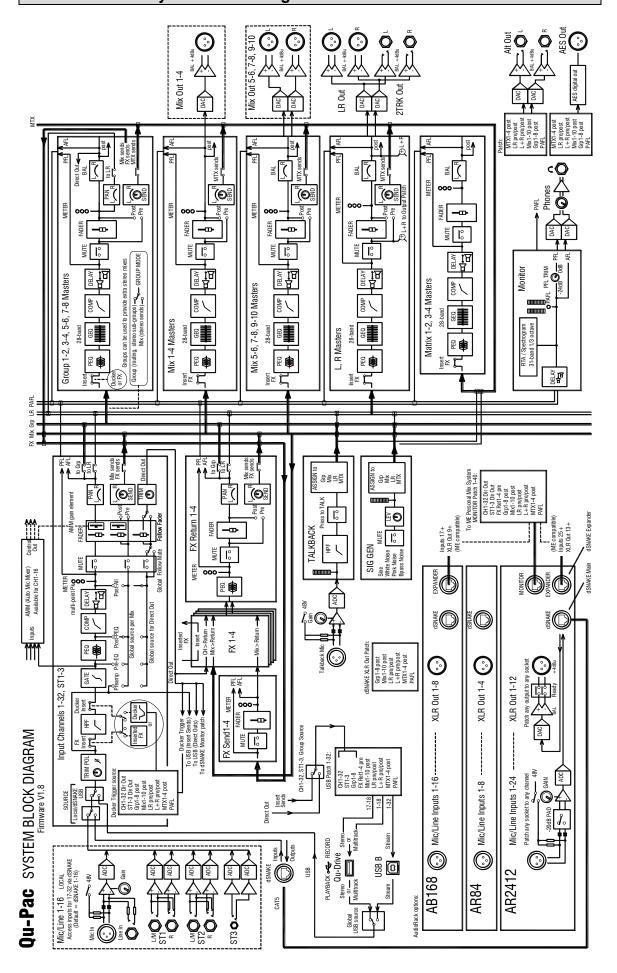
38 channel x 26 bus x 20 mix + 4FX DSP Engine
