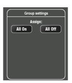
**Group Mode** - Touch the **Group** mode button to set operating mode as a stereo Audio Group. This provides routing that follows the channel pan control. You can assign combinations of channels and FX returns to a group. Groups can be routed to LR or any Mix to create sub-groups. Groups can be mixed to the Matrix (not available on Qu-16).
