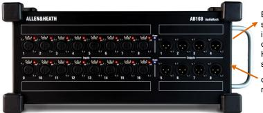
EXPANDER – To connect to a second AB168 to add more input and output sockets. Also compatible with the Allen & Heath ME personal mixing system.
