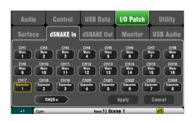
Use this screen to patch AudioRack input sockets to the Qu input channels. You can connect up to two AudioRacks via the dSNAKE Cat5 digital snake.
