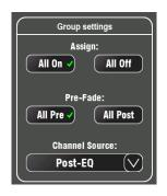
**Mix Mode** - Touch the **Mix** mode button to set operating mode as a stereo Mix. This provides channel send levels, dedicated pan, assignments, pre/post and source selection to the mix. You can assign combinations of channels, FX returns and groups to a mix. Mixes can be mixed to the Matrix.
