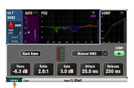
**Function Key** – The **Fn** key provides access to further options associated with the currently selected screen, for example channel source selection and processing libraries. It is also used to access the Mute Group and Matrix mix settings. If available, its function will appear in the lower toolbar above the key. Press the key again to close the option screen.
