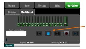
**Qu-Drive Multitrack page** – This screen presents the controls for multitrack recording to, and playback from a USB storage device plugged into the top panel Qu-Drive port.
