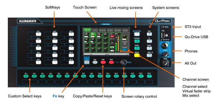
**Touch Screen** - All live mixing, setup and memory management functions can be controlled from the Qu-Pac front panel. The colour touch screen provides quick access to these functions. The top presents tabs for the available pages. The bottom presents a toolbar showing status information.
