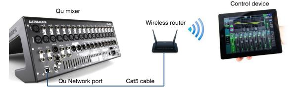
**Choosing a wireless router** - For best performance we recommend you use a dual band (2.4 and 5GHz) wireless router (wireless access point) with auto channel selection. A wireless router with auto channel selection automatically sets itself to an available or least congested channel when you power it up.
