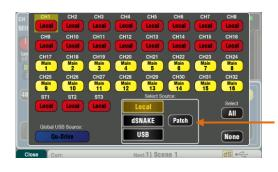
Inputs – Use the Preamp screen Fn key Source page to choose either the local (rear panel) socket or a remote (dSNAKE) socket for each channel source. Red buttons show local sources selected, yellow buttons show dSNAKE sources.
