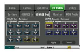
The following sources can be patched: Unassigned Grp Group post-fader Mix Mix 1-10 post-fader LR pre LR mix - pre-fader LR post LR mix - post-fader L+R pre LR mono sum - pre-fader L+R LR mono sum - post-fader MTX Matrix post-fader **PAFL** Stereo PAFL monitor
