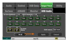
Stream audio to the computer – Audio is sent via the rear panel USB B port. Go to the Setup / Output Patch / USB Audio screen to choose which Qu outputs to patch to the USB stream.
