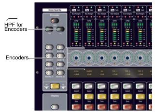
HPF controls for Input Channels
