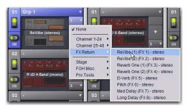
Assigning plug-in output to an FX Return
