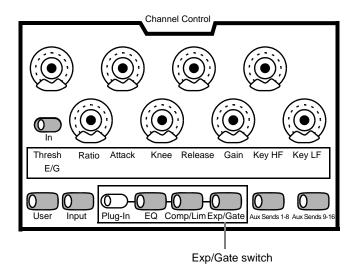
Expander/gate parameters in Channel Control
