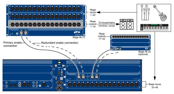
Figure 8. SC48 Remote Back panel and Stage 48 I/O slots and snake connectors
