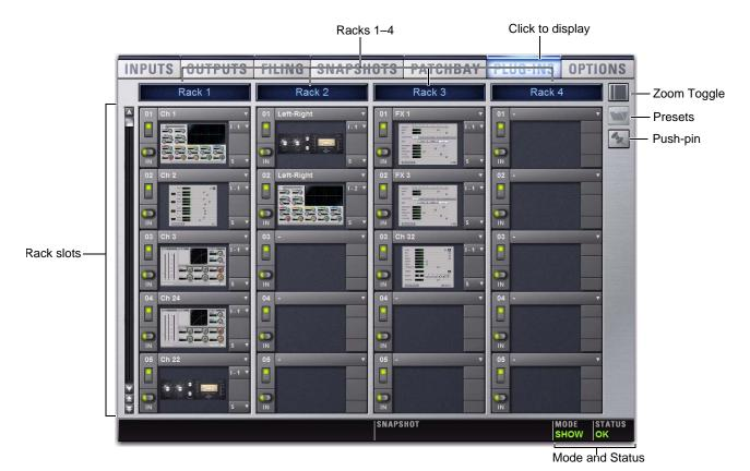
Figure 14. Plug-In racks and rack slots, Main view, with custom rack names shown.
