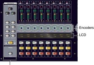
Encoder Assignment Switches Input encoders, assignment switches, and LCD (inputs 1–8)
