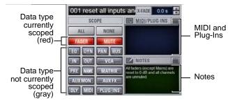
Data Type Scope buttons showing different scope states
