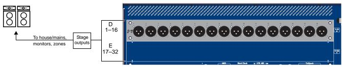
Figure 7. SC48 I/O slots D and E for stage Outputs 1-32
