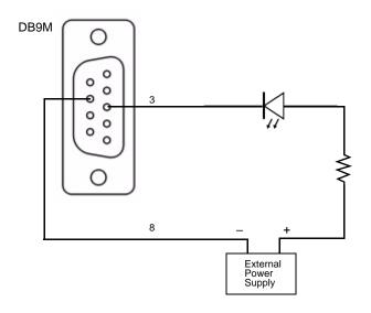
GPI Output Driving a Relay Using an External Power Supply
