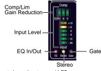
Input channel meters and LEDs
