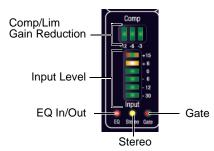
Input channel meters and LEDs
