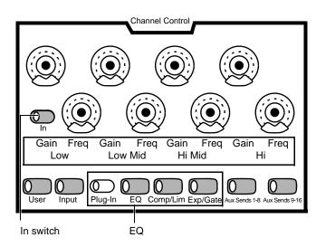
EQ controls in Channel Control (built-in 4-band shown)
