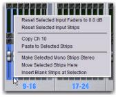
Two mono inputs about to be combined into one stereo channel
