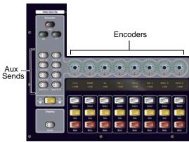
Encoder assignment switches for input channels
