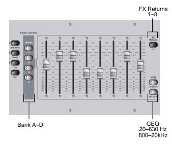
Input fader banking and assignment switches
