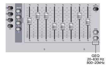
Input fader banking and assignment switches
