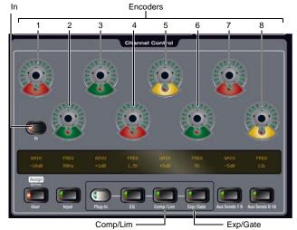
Controls for built-in dynamics processors in Channel Control
