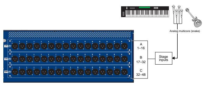
Figure 6. SC48 I/O slots A-C for stage inputs 1-48
