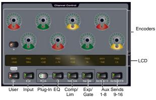
Channel Control encoders, LCD and mode switches
