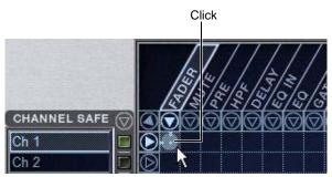
Enabling recall safe for channel 1 fader
