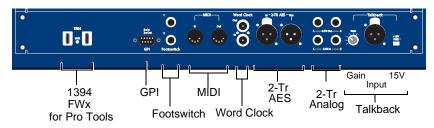
Figure 9. FOH connectors and controls
