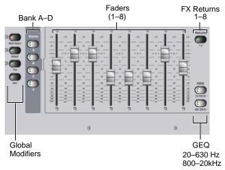
Input fader banking and assignment switches
