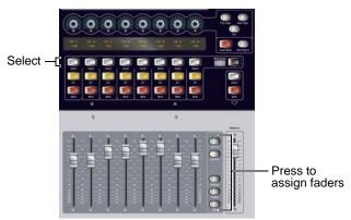
Bank switches for Output channels
