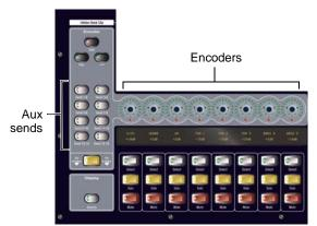
Encoder assignment switches for input channels
