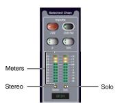
Selected Channel meters and LEDs
