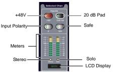
Selected Channel Input controls, meters and displays
