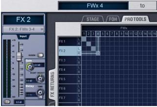
Patching FWx channels to FX Returns for playback
