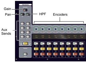
Encoder assignment switches for input channels
