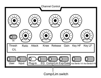
Compressor/limiter parameters in Channel Control
