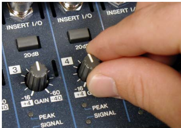
Figure 2-4 Setting console preamp gain
