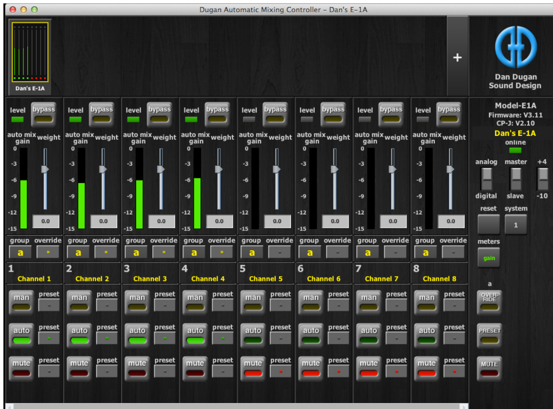
Figure 4-1 Dugan Control Panel
