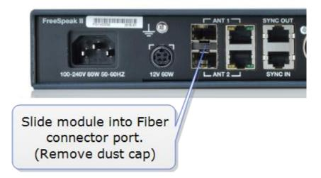
Install splitter Fiber module.
