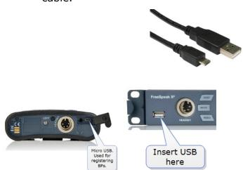
The beltpack can be powered on either before or after connection.
