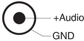
**Figure 9.** GT auxiliary equipment RCA jack
