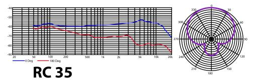
Large 1 1/2" diaphragm dynamic Type Frequency Response 40 Hz to 18 kHz
