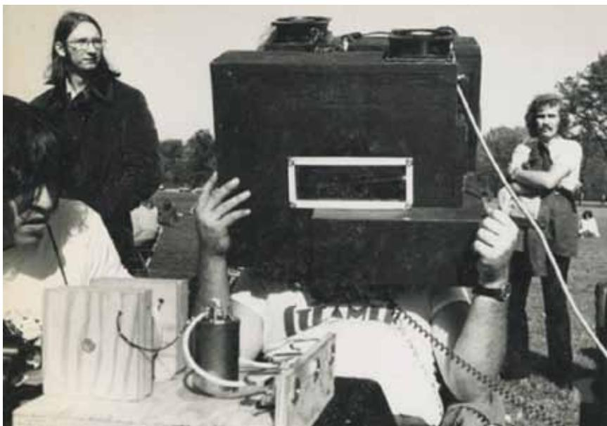
A "sound isolation helmet" circa 1974 that was designed, built, and deployed by the Steamer Sound team to isolate from the main system in order to mix on headphones for a live radio broadcast. Note the built-in "life support system" – boxer fans that would draw fresh air through the helmet to prevent suffocation and heat exhaustion.
