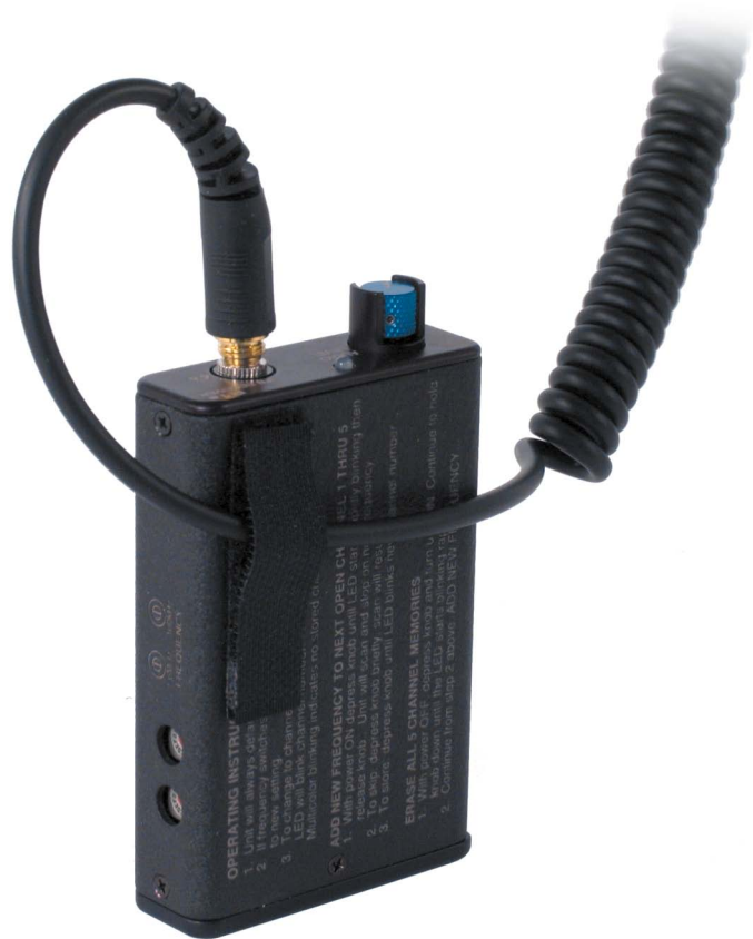
Figure 2 - Headphone cord strain relief
