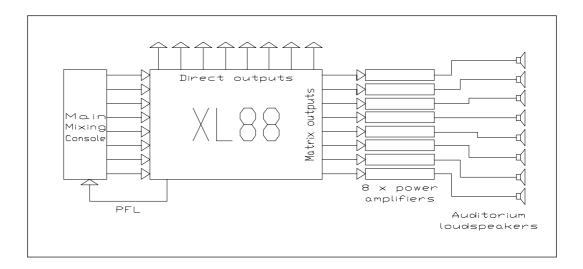
The large output faders give quick, precise, control over the output level to each loudspeaker, or group of loudspeakers. To pre-fade listen any input or output, the XL88's PFL output is brought back to a spare channel on the main console where the operator can monitor it on headphones simply by pressing the appropriate PFL button on the main console.
