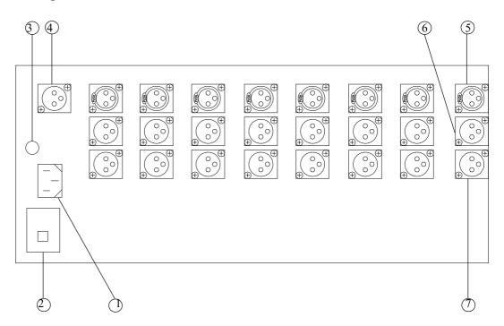
1) **Mains**. Supplied via an IEC standard 3-pin connector. A compatible power cord is supplied with the unit.
