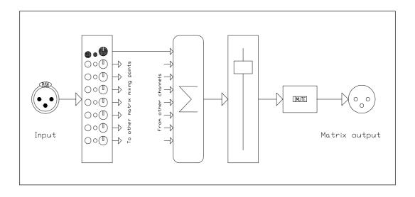
The eight Routing buttons on the input module are used to select which outputs the signal will be routed to. The eight Routing Level Controls adjust how much level is sent to each Matrix mixing point. Please note that these controls adjust the OUTGOING signal from the module.
