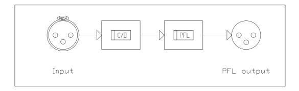
To Pre-Fade Listen to any input, leave the appropriate meter change over switch out and press the corresponding output PFL button whose
