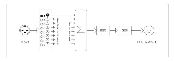
To Pre-Fade Listen any output, leave the Meter Changeover switch on the corresponding module out, the LED will be off, and press the Output PFL button whose associated red LED will light.
