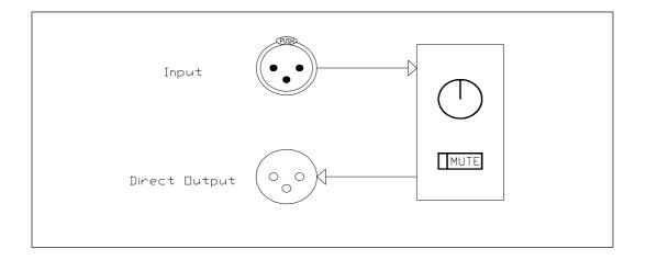
The Direct Output Level Control can vary the level from no signal to +10dB. The Direct Output Mute cuts the signal and is active when the button is depressed and the red LED glowing.
