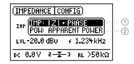
In the mode |Z| + Phase (1) the absolute value of the impedance and the phase is shown.
