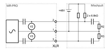
The most common phantom voltage is 48 V and lies on both Pin 2 and Pin 3 with balanced impedances (see diagram).
