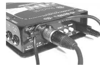
The JDV's strain relief in action.
