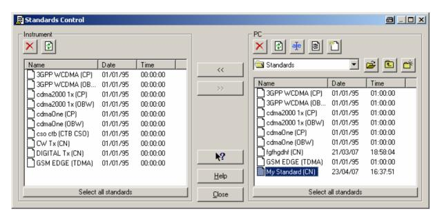
On the left side the standards are listed which are stored in the instrument. On the right side the standards are listed which are stored in the directory ...\Standards of the PC. Behind the standard name the measurement name is given in brackets. (CN) indicates a carrier / noise measurement standard.
