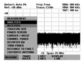
The R&S FSH activates the receiver mode and measures the level at the specified frequency.
