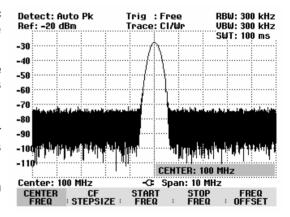
The smallest step for adjusting the center frequency with the rotary knob is a pixel, in other words, as the trace comprises about 300 pixels, each step is equal to about 1/300 of the span. When you use the cursor keys, a frequency step is equal to 10 % of the span (= 1 grid division). If you want to use a different step size, you can define it with the CF STEPSIZE function (CF = center frequency).
