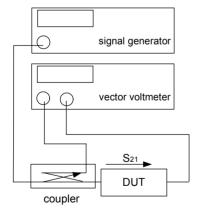
Fig. 3: Conventional test setup for transmission measurements using a vector voltmeter
