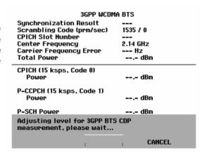
To demodulate the 3GPP signal, you must know the scrambling code (primary/secondary) of the base station. The scrambling code is either manually entered or automatically determined by the R&S FSH.
