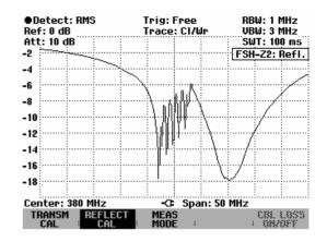
The reflection calibration remains valid until the R&S FSH's center frequency or span is changed such that the new span falls outside the calibrated frequency range. If calibration becomes invalid, the R&S FSH displays Uncal in the upper right-hand corner of the screen.
