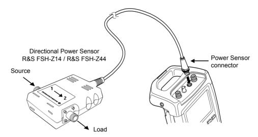
When measuring high powers, strictly observe the following instructions to prevent damage to the sensor or hazard to persons:
