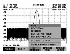
The R&S FSH allows you to use only a limited section of the trace for the PEAK, NEXT PEAK and MINIMUM functions. This is beneficial, for example, if you want to sample only spurious emissions with the marker search functions and want to omit useful signals.
