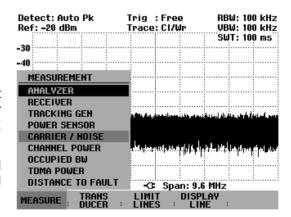
The most important measurement parameter settings are available directly in the main menu of the carrier/noise measurement or can be entered using the corresponding function keys.
