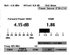
To ensure that true results are output when measuring modulated signals, the R&S FSH offers the possibility of taking correction values into account for a number of common transmission standards.
