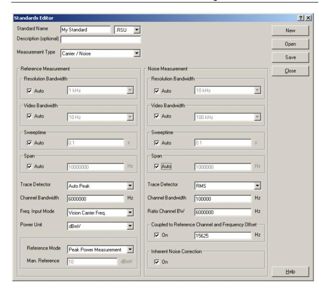
The standard settings are stored in the PC and can be transferred and stored to the instrument R&S FSH via the PC cable.
