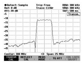
The transmission calibration remains valid until the center frequency or the span is changed on the R&S FSH such that the new span falls outside the calibrated frequency range. If the calibration is no longer valid,. Uncal is displayed in the upper right-hand corner of the screen.
