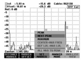
The resolution of cable faults can be increased by a zoom function. This is used primarily with long cables to better distinguish faults that are very close to each other.
