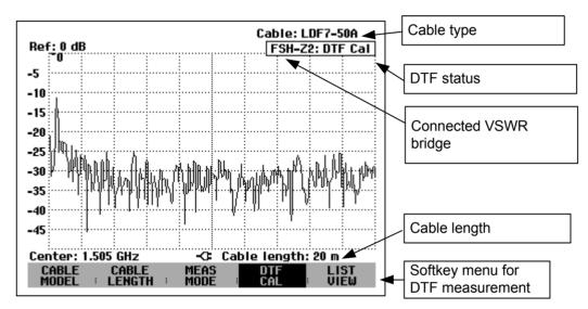
To perform distance-to-fault measurements, the R&S FSH needs to "know" the type of cable and its approximate length.
