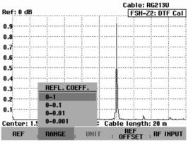
The R&S FSH can also list any cable faults. It displays the return loss and distance from the measurement plane of all reflections that exceed a settable threshold.
