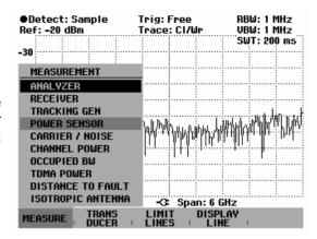
The R&S FSH opens the screen for power measurements. If no power sensor is connected, no measured value is displayed. If a power sensor is connected, the R&S FSH sets up a connection via its interface and after a few seconds displays the measured power.
