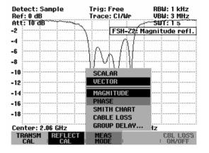
The R&S FSH displays the DUT's phase characteristic as a function of the frequency. Phase refl. will appear in the upper right-hand corner of the display. In the default scaling, the phase can only have values between -180° and +180°.
