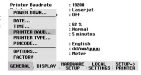
The selection box for the available baud rates (1200 baud to 115 200 baud) opens.
