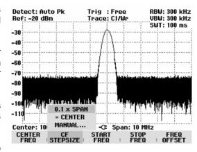
If you select "0.1 x SPAN" or "= CENTER", the R&S FSH makes the setting directly itself. If you select "MANUAL...", the value entry box opens and indicates the current step size.
