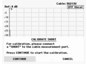
When calibration is over, the R&S FSH displays DTF CAL in the upper right-hand corner of the screen.
