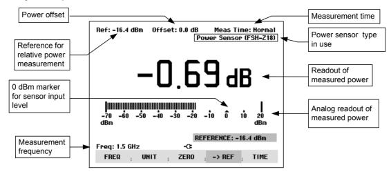
The power sensor has a memory containing frequency-dependent correction values. This means that the highest accuracy is reached for signals whose frequency is known. If the R&S FSH switches over to the power measurement mode from another operating mode, it uses the center frequency as the frequency for the power sensor.
