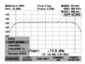
If USER is selected, the R&S FSH sets the last channel power measurement setting used in the USER mode. The R&S FSH automatically makes changes to the setting so that it is again available when the USER standard is called again.
