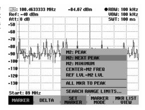
In addition, it is possible to position all activated markers (M1 to M6) at the peak of a trace.
