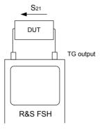
Fig. 4: Test setup for transmission measurements using the R&S FSH
