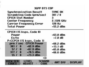
In the case of base stations with two antennas, you must specify which of the antennas to synchronize to. For base stations with only one antenna, the default value is OFF.
