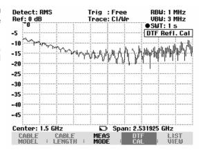
Checking the spectrum in the span for detecting external interferers:
