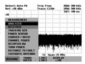
The R&S FSH activates the receiver mode and measures the level on the set frequency.
