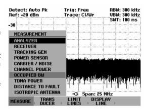
The R&S FSH displays the softkey menu for setting the measurement of occupied bandwidth. Two vertical lines in the measurement diagram indicate the occupied bandwidth. The measured numeric value (OBW) is shown in large characters below the measurement diagram.
