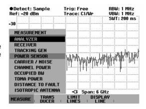
The R&S FSH opens the screen for power measurements. If no power sensor is connected, it does not display any measured value and outputs Power sensor (unknown) in the status field. If a power sensor is connected, the R&S FSH sets up a connection via its interface, displays first the message Power sensor (Detecting) and then the message Power sensor (Booting) in the status field and, after a few seconds, displays the type of the sensor connected (R&S FSH-Z44) as well as the measured power.
