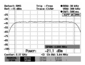
The largest permissible span for the channel power measurement is ten times the channel bandwidth. At larger spans, the result of the channel power measurement would be increasingly imprecise, because too few points of the trace occur in the channel to be measured.
