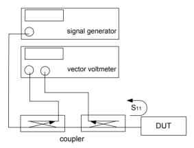
Fig. 1: Conventional test setup for reflection measurements using a vector voltmeter
