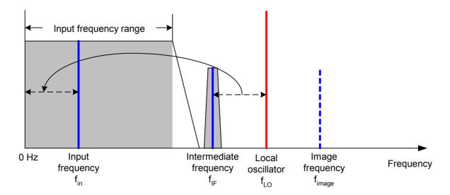
The first local oscillator is tuned with a sawtooth which simultaneously acts as the x deflection voltage for the display. In practice, synthesizer technology is used to generate the frequency of the first local oscillator and for a digital display.
