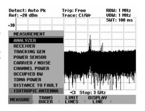
The R&S FSH will open the measurement function menu and activate the Isotropic Antenna measurement function. Before displaying final measurement results, the R&S FSH performs a measurement for each of the three antenna axes so that the update rate of the trace decreases accordingly.
