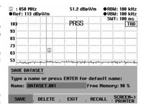
The data set name comprises a text section and a numeric extension, which are separated by a full stop. The data set name suggested by the R&S FSH is derived from the name of the data set last stored, the numeric extension being incremented by 1 in each case.
