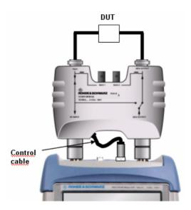
As soon as the control cable has been connected to the R&S FSH, the VSWR Bridge R&S FSH-Z3 is automatically detected and indicated both on the display and the status menu. Automatic detection requires that this feature be activated in the SETUP menu (default setting). See also "Settings for detection of the R&S FSH-Z3 in transmission and spectrum measurements".
