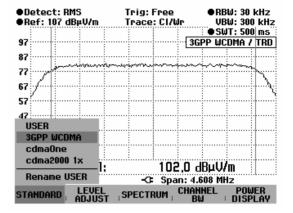
If you select USER, the R&S FSH will restore the channel power measurement setting last used with USER. It automatically incorporates changes in the settings so that they will also be available the next time the USER standard is called.
