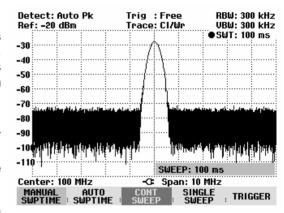
Whenever a change is made, the sweep time is immediately set to its new value. The value entry box is closed by pressing the ENTER key. The sweep time that has been set is displayed in the upper right-hand corner of the screen in the SWT readout box.
