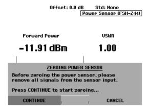
The R&S FSH immediately starts power sensor zeroing. While this is being done, the R&S FSH outputs the message "Zeroing power sensor, please wait...".
