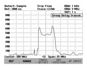
Defining the span for the group delay measurement:
