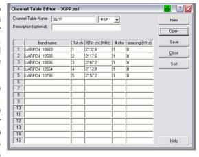
➤ After the channel list has been selected, the R&S FSH can be set in turn to each center frequency associated with a channel number in the list using the rotary knob or the arrow keys. (see Chapter "How to Use Channel Tables")
