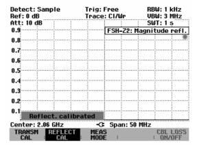
The reflection calibration remains valid until the center frequency or the span is changed on the R&S FSH to such an extent that the new span falls outside the calibrated frequency range. Uncal is displayed in the upper right-hand corner of the screen when calibration is no longer valid.
