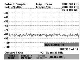
If the sweep is continuous, the R&S FSH then performs a sliding averaging. In the SINGLE SWEEP mode, it performs exactly those sweeps defined with AVG COUNT and averages the traces. It then stops the sweep and displays the averaged trace.
