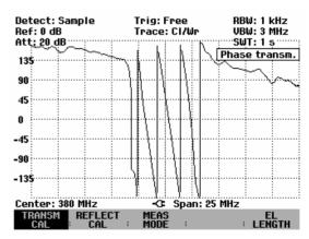
The UNWRAP function removes the restriction limiting the value range to ±180°. With this function, no more shifts will occur, and the phase can have any value from 0° to 54360°. You can activate the UNWRAP function as follows:
