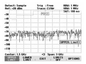
All active limit lines can be switched off together with the LIMITS OFF softkey.
