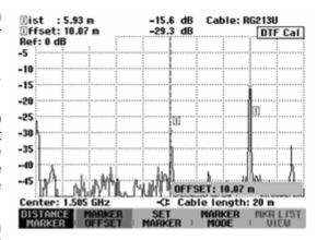
As is the case with spectrum analysis, the R&S FSH provides functions to automatically position the marker or the marker offset on the trace. These can all be accessed by pressing the SET MARKER softkey.
