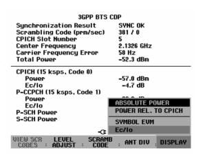
The channel powers of P-CCPCH, P-SCH and S-SCH can also be displayed as relative powers with respect to the CPICH channel.
