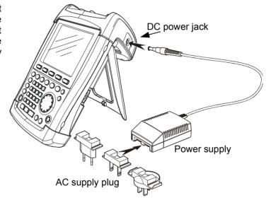
For rapid charging, be sure to switch off the R&S FSH during charging. The charging time is approx. seven hours. After four hours, the battery will be approx. 80 % charged.
