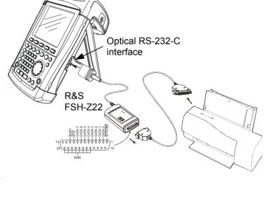
While data is being transmitted to the printer, the "Busy" LED remains lit.
