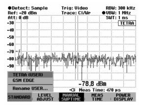
Using the R&S FSH View control software, additional standards can be generated and permanently loaded into the R&S FSH. You can also delete the factory-set standards provided in the instrument if you do not need them. The R&S FSH then offers only the standards you require.
