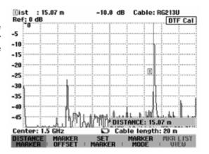
For higher fault resolution, the R&S FSH offers a zoom function in the position of the marker. The x axis of the display can be extended up to a span of 3 m.
