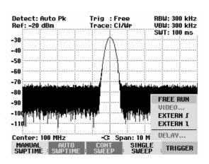
If the VIDEO... trigger setting has been selected, the trigger level and any trigger delay (DELAY...) must be entered. The trigger level is expressed as a percentage (%) of the reference level. 100 % means that the trigger level equals the reference level, 50 % that the trigger level is in the middle of the y axis on the measurement diagram (default setting). The position of the video trigger on the level axis is shown by a ">".
