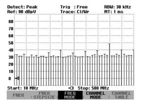
Pressing the FIXED FREQ softkey switches the R&S FSH back to the default setting of the receiver mode.
