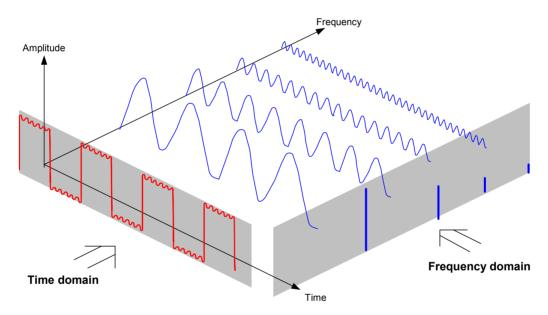
The periodic squarewave in the time domain can be Fourier transformed to the frequency domain. In the case of a squarewave there is a fundamental (= frequency of the squarewave) and its odd harmonics. Using a narrow bandpass filter, the spectrum analyzer makes measurements in the frequency domain. Only at frequencies where there is a signal is there a reading which gives the amplitude of the frequency component.
