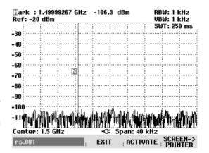
Pressing the ACTIVATE softkey transfers the stored trace to the R&S FSH's trace memory. The current trace can be compared with the stored one by switching on the trace memory.
