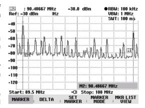
The R&S FSH displays the marker or delta marker last edited in the marker readout box at the upper left-hand corner of the screen. All marker functions in the SET MARKER menu apply to the displayed markers.
