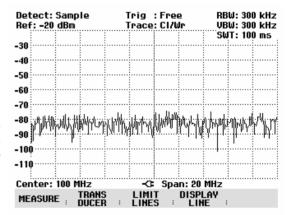
The R&S FSH makes a distinction between upper limit lines (UPPER LIMIT) and lower limit lines (LOWER LIMIT). It checks whether a measured value is above the upper limit line or below the lower limit line. The limit lines stored in the R&S FSH can be used to mark both upper and lower limit values.
