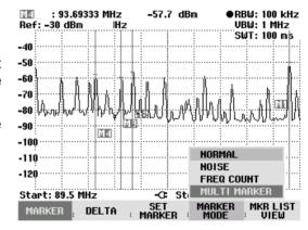
The R&S FSH transfers the settings of the multimarker and multi delta marker with the lowest numbers to the normal marker mode.
