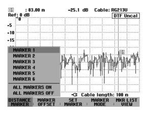
After a marker is activated, its position is indicated in the value entry box. To vary the marker position, use the number keys to enter a distance (e.g. 11.5 m), or move the marker pixel by pixel with the rotary knob, or move it in steps of 10% of the displayed cable length by means of the cursor keys. For fast marker positioning, it is recommended that first coarse adjustment be performed with the cursor keys, and then fine adjustment with the rotary knob.
