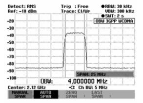
The largest permissible span for measuring the occupied bandwidth is ten times the channel bandwidth. At larger spans, the result of the channel power measurement would be increasingly imprecise, because too few points of the trace occur in the channel to be measured.
