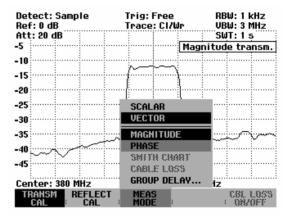
The R&S FSH displays the DUT's phase characteristic as a function of the frequency. Phase transm. will appear in the upper right-hand corner of the display. In the default scaling, the phase can only have values between -180° and +180°.
