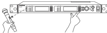
3. The display indicates if the IR sync is successful. Check transmitter alignment and select **Retry** if a failure occurs. The receiver passes an audio signal if successful.
