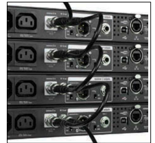
RF distribution ports allow up to 10 receivers to share a single pair of antennas.
