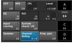
Channel linking example: EQ A  $\ P$  B; EQ and Delay C  $\ P$  D
