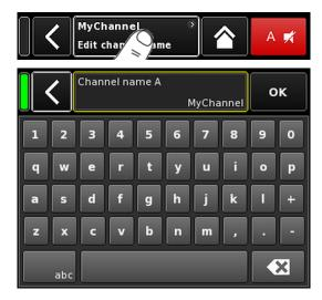
Selecting a particular channel from the Home screen opens the corresponding Channel setup screen with the respective Channel tab being active.
