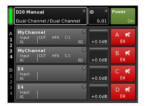
From the Home screen, the menu structure of the operating software is divided into two main axes, the Device setup and the Channel setup. The navigation buttons allow for direct vertical access to the specific submenus while the tab structure on the right side of each submenu provides a clear horizontal order.
