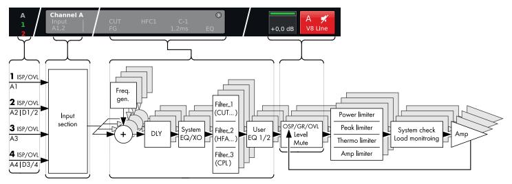
D20 Channel strip block diagram (signal chain)
