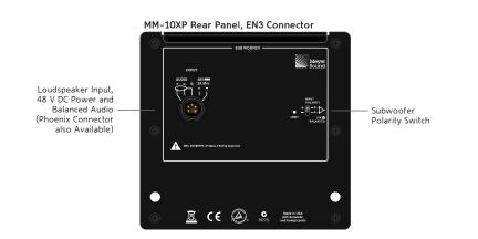
The loudspeaker shall be equipped with either a Phoenix 5-pin male or EN3 5-pin male connector (three pins for balanced audio and two pins for DC power). The audio input shall be electronically balanced with a 10-kOhm impedance and accept a nominal -2.0 dBV (0.8 V rms, 1.1 V peak) input signal. DC blocking and RF filtering shall be provided, and CMRR shall be greater than 50 dB and typically 80 dB (50 Hz to 500 Hz).
