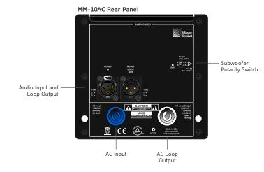
The audio input shall be electronically balanced with a 10-kOhm impedance and accept a nominal -2.0 dBV (0.8 V rms, 1.1 V peak) input signal. Connectors shall be XLR female for input and XLR male for loop output. DC blocking and RF filtering shall be provided, and CMRR shall be greater than 50 dB and typically 80 dB (50 Hz to 500 Hz).
