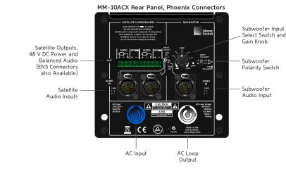
The audio input shall be electronically balanced with a 10-kOhm impedance and accept a nominal -2.0 dBV (0.8 V rms, 1.1 V peak) input signal. Three XLR female input connectors shall be provided, one for the subwoofer and two for satellite loudspeakers. DC blocking and RF filtering shall be provided, and CMRR shall be greater than 50 dB and typically 80 dB (50 Hz to 500 Hz). Two output connectors shall be provided for routing balanced audio and 48 V of DC power to the satellite loudspeakers.
